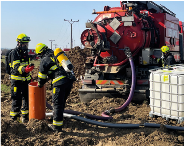
Pumping pure benzene into a specialized hazardous waste tank of the Firefighters Decontamination Unit
