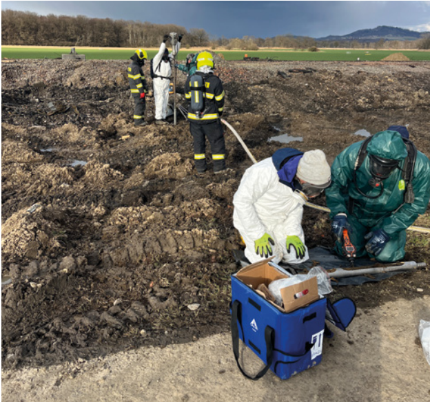
Establishment of dug probes and simultaneous measurement of benzene levels in the air
